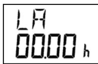
Display of the time that has elapsed since the start of the night-time charge release (start of charge release/LF)
