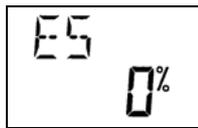
Changes to the basic charge level of all storage heating systems connected to the charge control. The set charge can be either proportionally raised or lowered by up to 30%, according to need. The change to the charge level should only be made gradually, since the effect of these changes will only become apparent after the unit has been charged.
